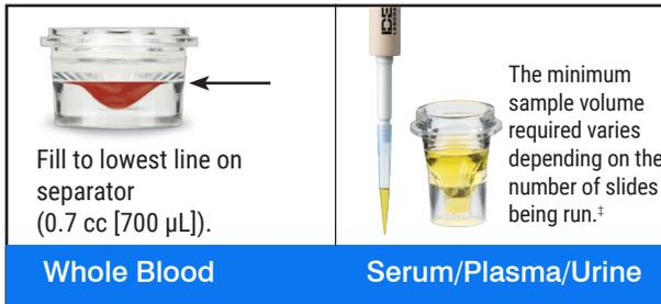
‡300 µL is the recommended sample volume when running a Chem 17 CLIP and electrolytes.
