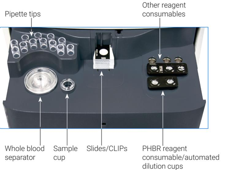
†The sample drawer photo (shown at right) is for reference purposes only. Not all consumables should be loaded for a single run (for example, never load both a whole blood separator and a sample cup).
