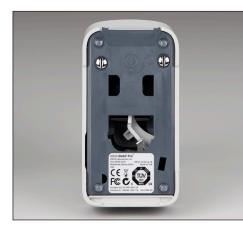
8. Ensure the base and silver fasteners are flush with the analyser and locked into place. Not locking the base and fasteners properly can impact analyser performance.
