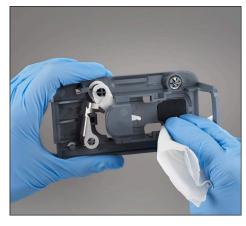
Clean the entire base using a lint-free wipe or cotton swab dampened with 70% isopropyl alcohol, mild liquid soap and water, or a 10% bleach solution.
