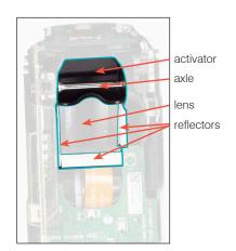
c. Clean the 3 white reflectors, the axle, and the activator using a new lint-free wipe or cotton swab dampened with 70% isopropyl alcohol, mild liquid soap and water, or a 10% bleach solution.
