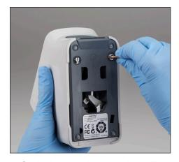
On the bottom of the switched-off analyser, use a flat-tip screw driver or coin to turn the 2 silver fasteners counterclockwise a quarter turn.
