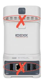
**DO NOT** wipe the vents underneath the power button or the USB/power/Ethernet ports.
