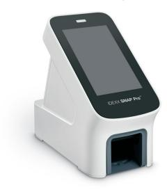
Clean the case and screen using a lint-free cloth dampened with 70% isopropyl alcohol, mild liquid soap and water, or a 10% bleach solution.
