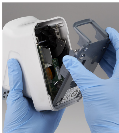
6. After the base has dried, reattach it to the analyser and ensure it is locked into place.
